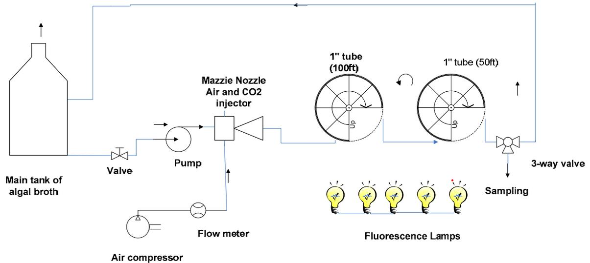
Figure 1: Tubular Photobioreactor
