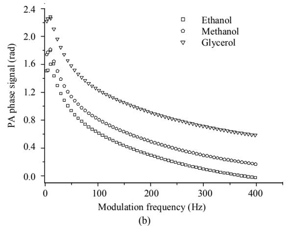
Fig. 2: The Photoacoustic signals as a function of the modulation frequency for the ethanol, methanol and glycerol. (a) Photoacoustic amplitude signal. (b) Photoacoustic phase signal
