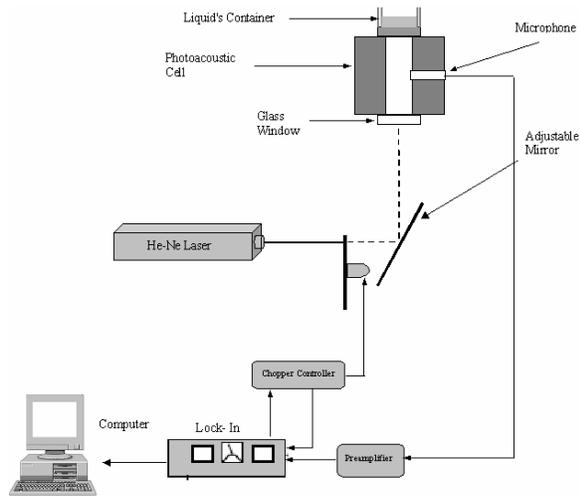
Fig. 1: Experimental setup of open photoacoustic technique
