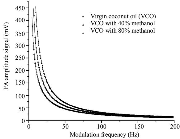
Fig. 3: The photoacoustic signal as a function of the modulation frequency for virgin coconut oil and coconut oil-mixture
