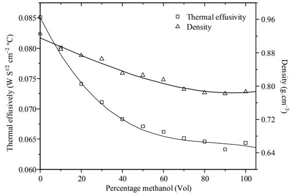
Fig. 4: Thermal effusivity and density measured at room temperature as a function of methanol in the solution
