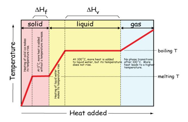
Let's trace that curve from left to right across five regions. Note that on the bottom axis we're just adding heat to the sample at a steady rate, but what is happening to the temperature is anything but steady.
