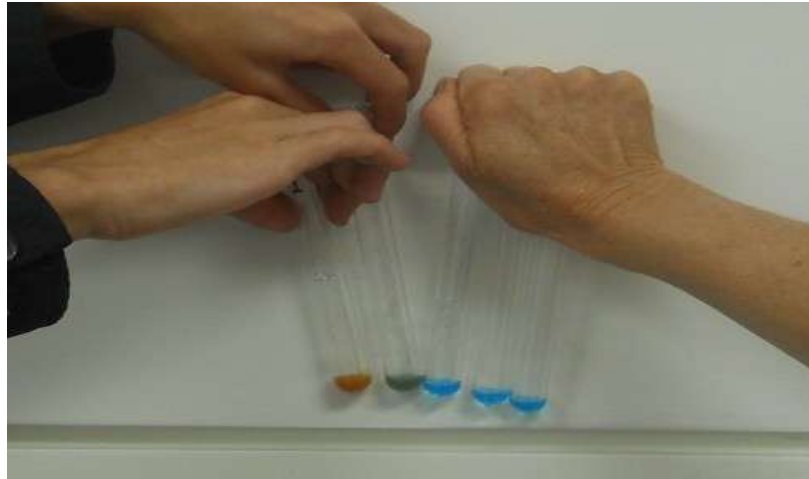
Figure 1. Testing for sugar using Benedict's solution. The test tube on the left indicates the presence of simple sugar, while the three on the right show none.
