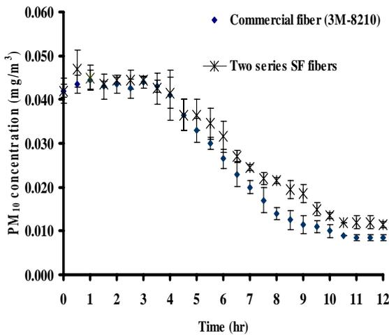
Fig. 5 PM<sub>10</sub> concentration before and after treatment at air flow rate of 5 L/min
