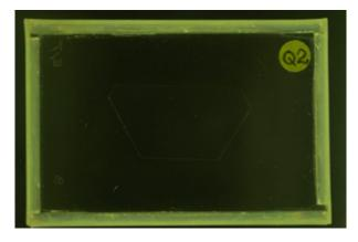
When the quartz sample is cut so that the incident light is parallel to the optic axis, no light is transmitted in any orientation.
