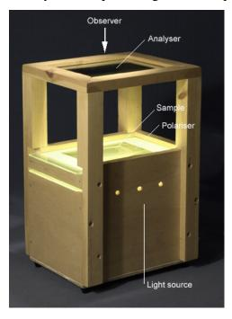
The apparatus used for examining optical anisotropy consists of a white-light source, two polarising filters and a frame to hold them apart so creating a working space.
