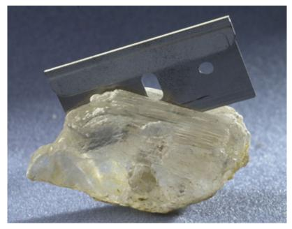
Certain crystals, such as gypsum, can be cleaved with a razor blade along particular crystallographically-determined planes.
