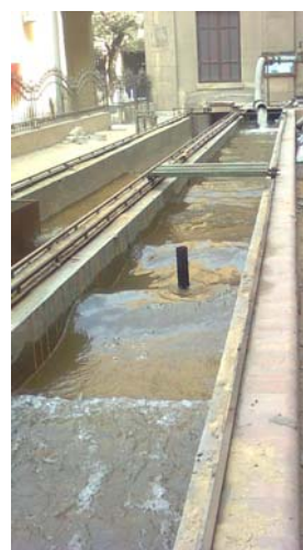
Figure 1. The flume used in this study showing the case of waves advancing against current. a) Section elevation and plan, b) Illustrative photo of the flume
