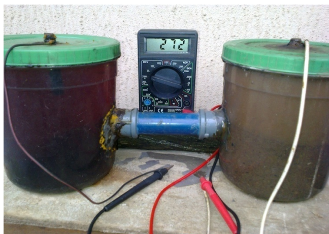
Figure 3 Experimental set-up for a dual chamber Microbial Fuel Cell (MFC)
