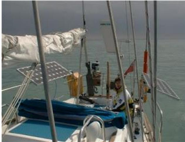
*The solar panels on this small yacht at sea can charge the 12 volt batteries at up to 9 amperes in full, direct sunlight.*
