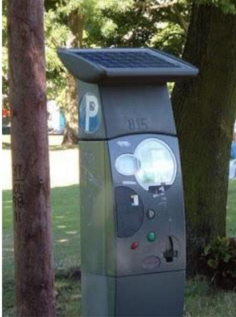
*A solar panel on top of a parking meter. Note that this particular installation is shaded, and may not perform as desired.*
