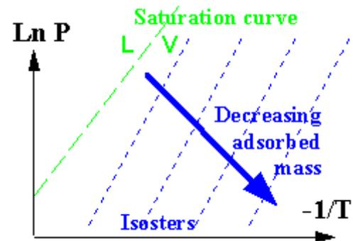
An adsorption cycle for refrigeration -or heat pumping- does not use any mechanical energy, but only heat energy. Moreover, this type of cycle basically is a four temperature discontinuous cycle.
