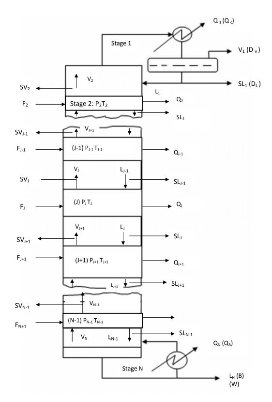
Fig. 26.1: Continuous Distillation Column
