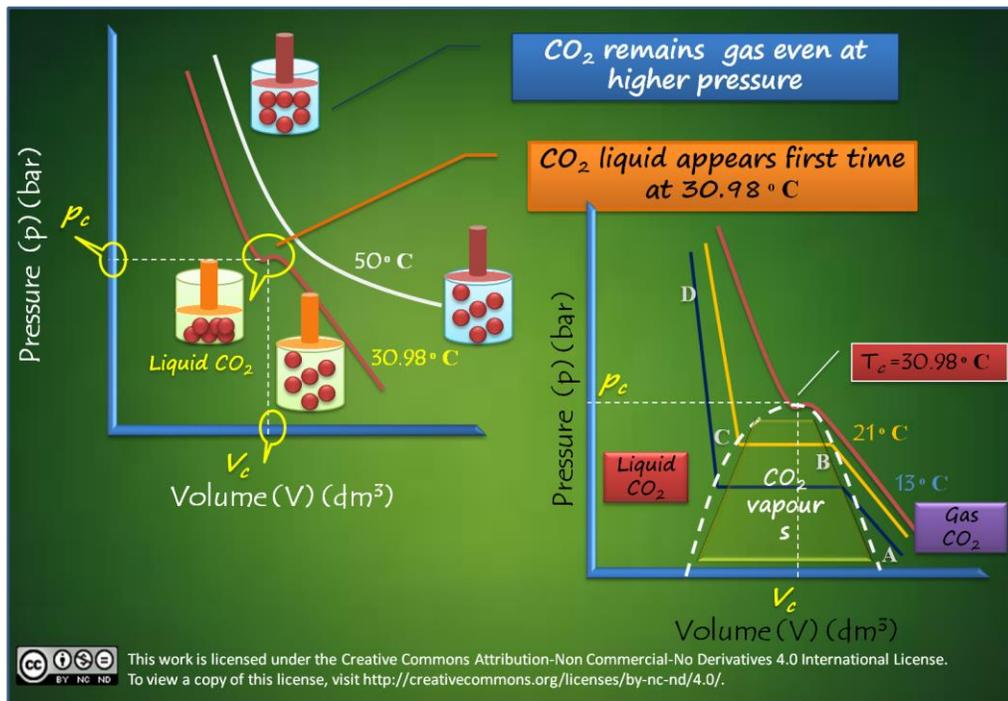
**What happens if we further reduce the temperature?** CO<sub>2</sub> gas shows different behaviour on applying pressure at temperature below 30.98°C.
