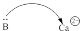
Figure AB3.4. A calcium ion essentially has a noble gas configuration. Nevertheless, its positive charge can attract electrons from a donor atom.
