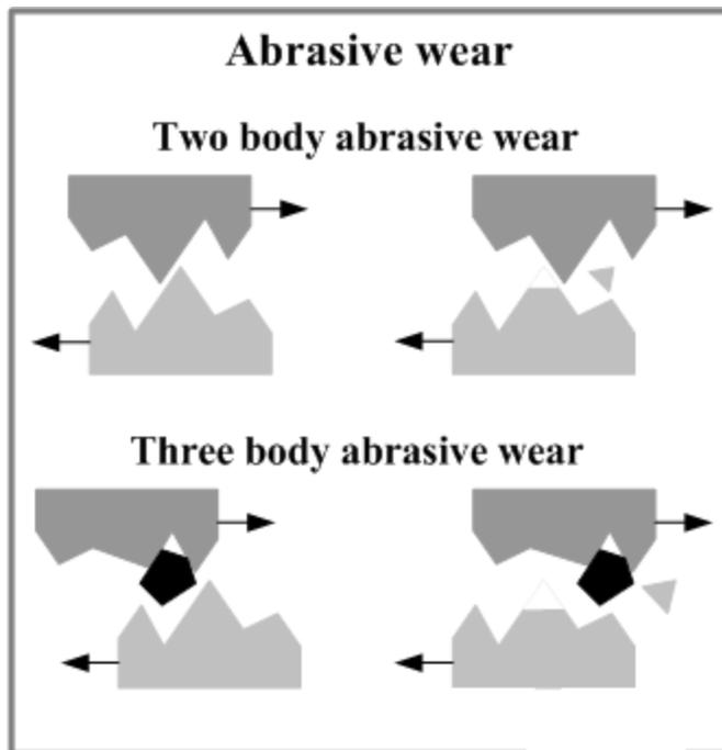
**Fig.2 Abrasive wear**
