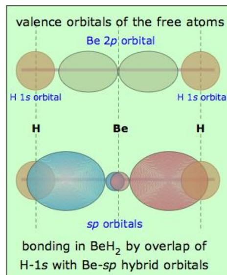
Notice that whereas a single p-orbital has lobes on both sides of the atom, a single sp-hybrid has most of its electron density on one side, with a minor and more spherical lobe on the other side. This minor lobe is centered on the central atom (some textbook illustrations don't get this right.)
