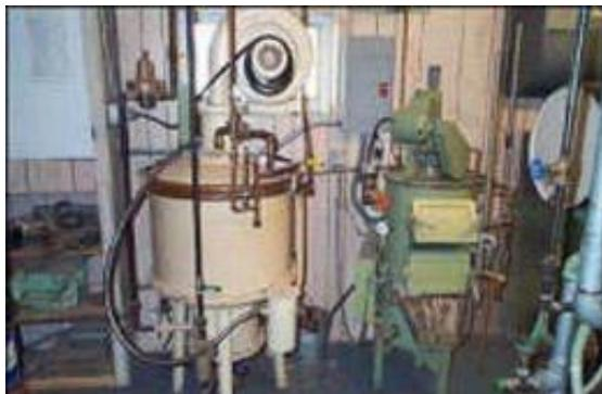
Tetrachloroethylene tankage used in dry-cleaning
