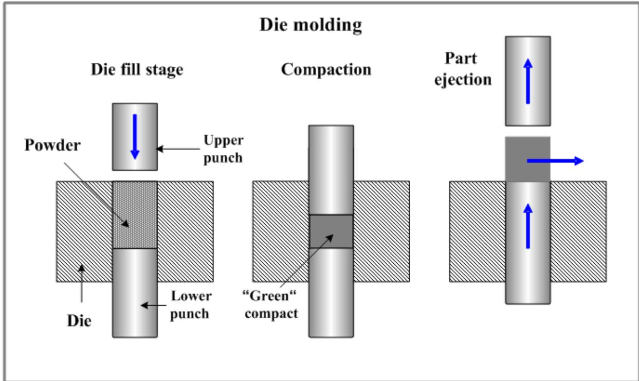
The die molding process consists of the following stages:
