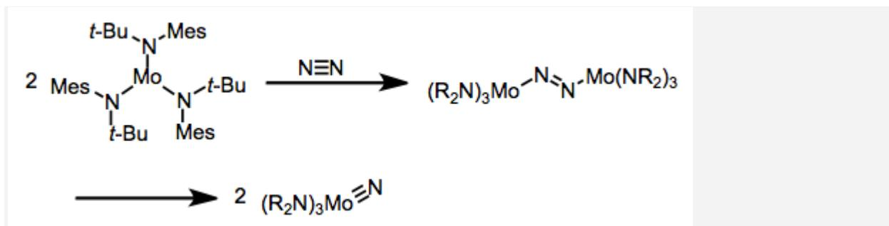
Activation of dinitrogen by molybdenum—a complex containing an "end-end," linear bridging dinitrogen (not shown) is proposed as an intermediate in this mechanism.
