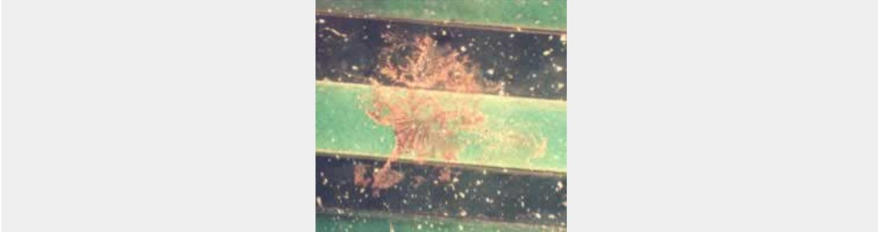
The rate of electromigration increases with temperature and has four prerequisites – a mobile metal; a voltage gradient; a continuous film of moisture; soluble ions:
