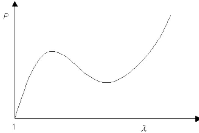
Although the tension in the balloon only ever rises with  $\lambda$ , it can be seen that this is not the case with pressure. The fact that there are regions of the graph for which
