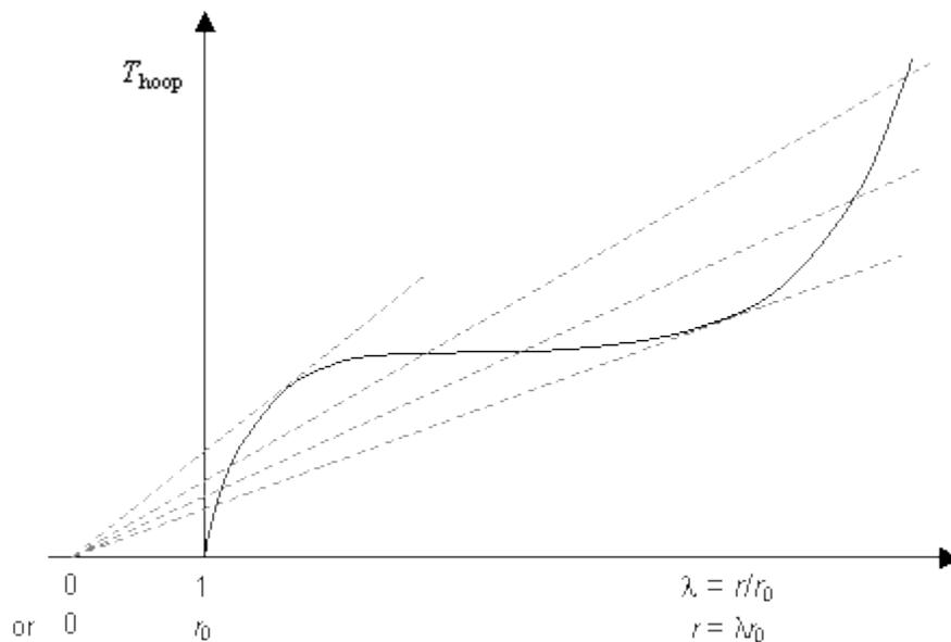
The gradients of the dashed lines are proportional to the pressure inside the balloon at the values of extension ratio (or radius) at which they cross the curve. This allows us to obtain the curve showing the variation of pressure with extension ratio:
