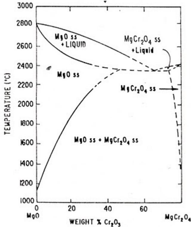
Fig: MgO-MgCr<sub>2</sub>O<sub>4</sub> binary Phase Diagram
