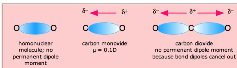
The zero dipole moment of CO<sub>2</sub> is one of the simplest experimental methods of demonstrating the linear shape of this molecule.
