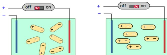
Measurement of the capacitance of a gas or solution is easy to carry out and serves as a means of determining the magnitude of the dipole moment of a substance.
