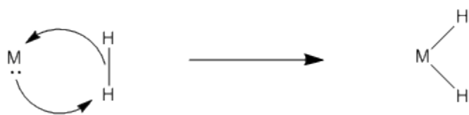
Figure OA4.3. A curved arrow representation of non-polar oxidative addition.
