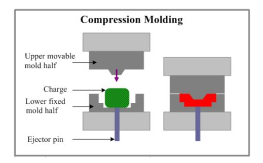
Compression Molding cycle time is about 1-6 min, which is longer than Injection Molding cycle. The method is suitable for molding large flat or moderately curved parts.
