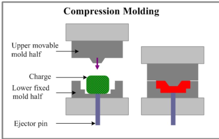
Compression Molding cycle time is about 1-6 min, which is longer than Injection Molding cycle.
