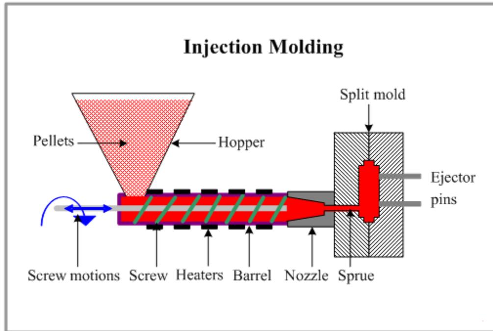
Injection Molding is highly productive method providing high accuracy and control of shape of the manufactured parts. The method is profitable in mass production of large number of identical parts.
