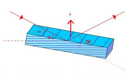
To measure the diffraction peak the sample is rotated by the offset. Now  $\omega$  is not equal to  $\theta$ . This is called an asymmetric reflection
