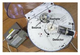
Top view of diffractometer (Click on image to view larger version)
