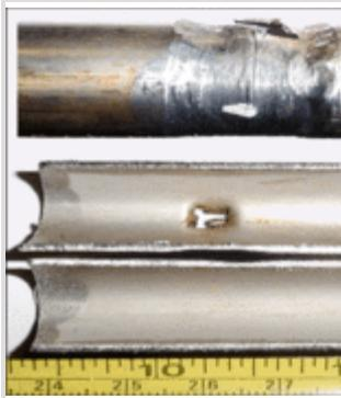
Figure 5: Flow-Induced Localized Corrosion
