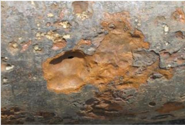
Figure 3: Pitting Corrosion
