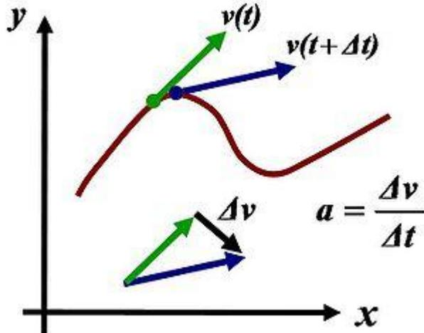
Figure 2. Components of acceleration for a planar curved motion.
