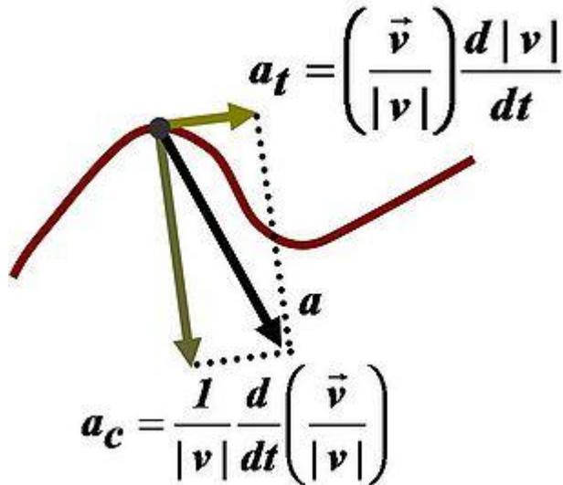
Figure 2. Components of acceleration for a planar curved motion.
