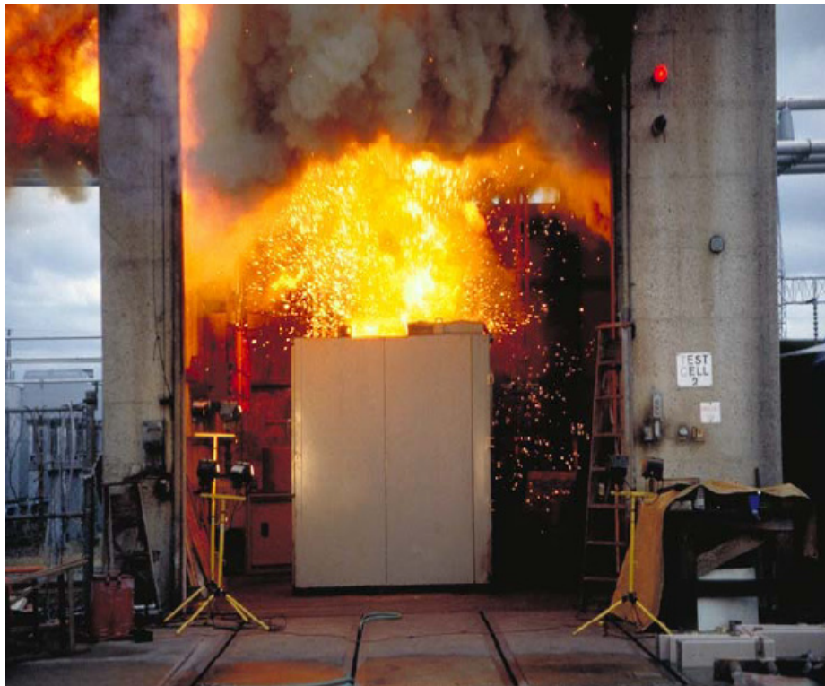
Figure 1.3 (a) Arc flash light and sound effects (photos taken from e-web engineering)
