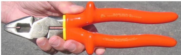
Picture 2: Insulated hand tool to IEC 60900 with an orange over yellow substrate
