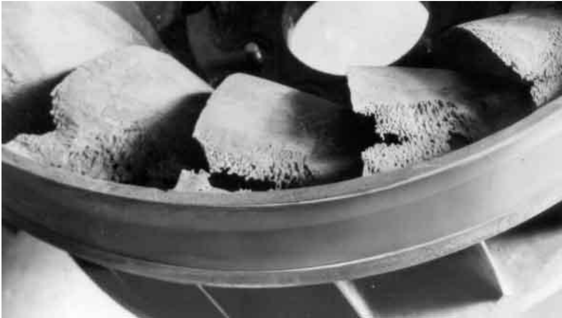
Figure 1: Cavitation damage to impeller blades (Image courtesy of California Institute of Technology)
