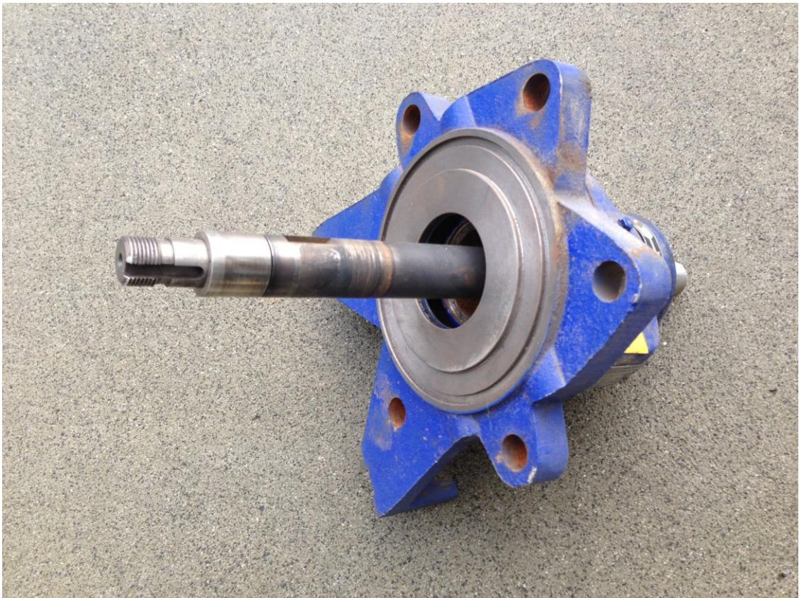
Figure 2: Damaged pump shaft after pump overheated due to lack of liquid
